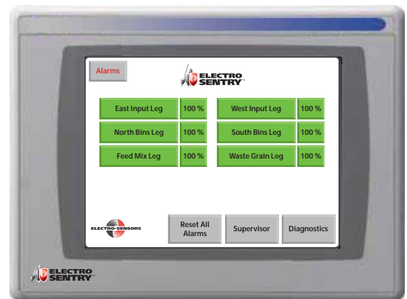
Normal Operation "Home" Screen View — No Alarms
