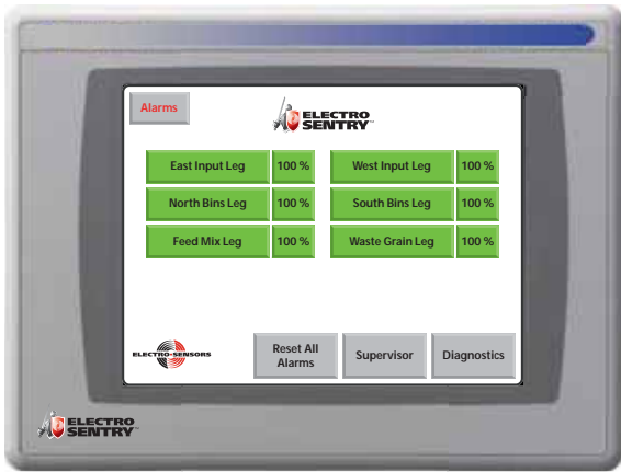
Normal Operation "Home" Screen View — No Alarms
