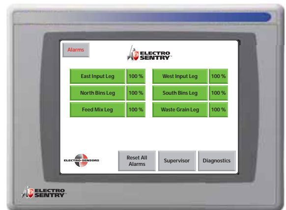
Normal Operation "Home" Screen View — No Alarms
