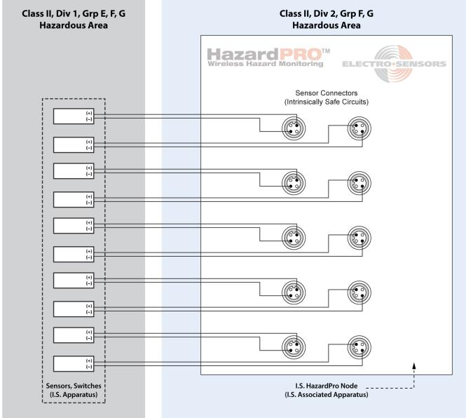
Interconnection of I.S. HazardPRO Node and each intrinsically safe apparatus shall satisfy the following:
