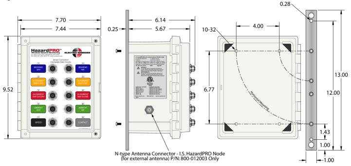
Each node comes with 2 aluminum mounting brackets and 4 (10-32) screws to attach them to the Node.
