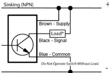
**Note:** When this sensor is used as a stand alone pulse generator, an external pull up resistor(\*) must be applied across the output as shown.
