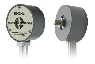
Minnetonka, MN-Electro-Sensors, Inc. announces the release of the EZ-3/4in and EZ-18mm Easy Mount Bracket Assemblies, which are used with Electro-Sensors speed sensors to generate pulses or 4-20 mA signals for use with display meters, speed switches, or PLC inputs. The EZ-18mm and EZ-3/4in easily mount directly into the tapped shaft so no other mounting brackets are needed.
