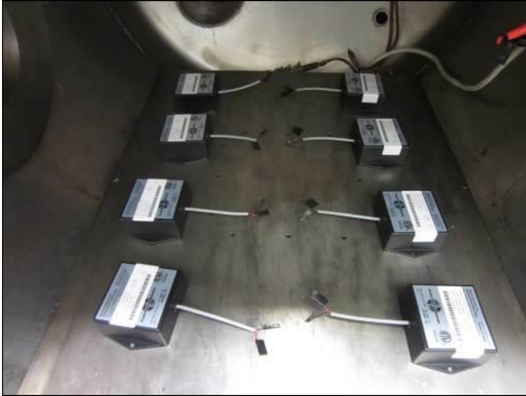
Photograph 1: Altitude Simulation Setup
