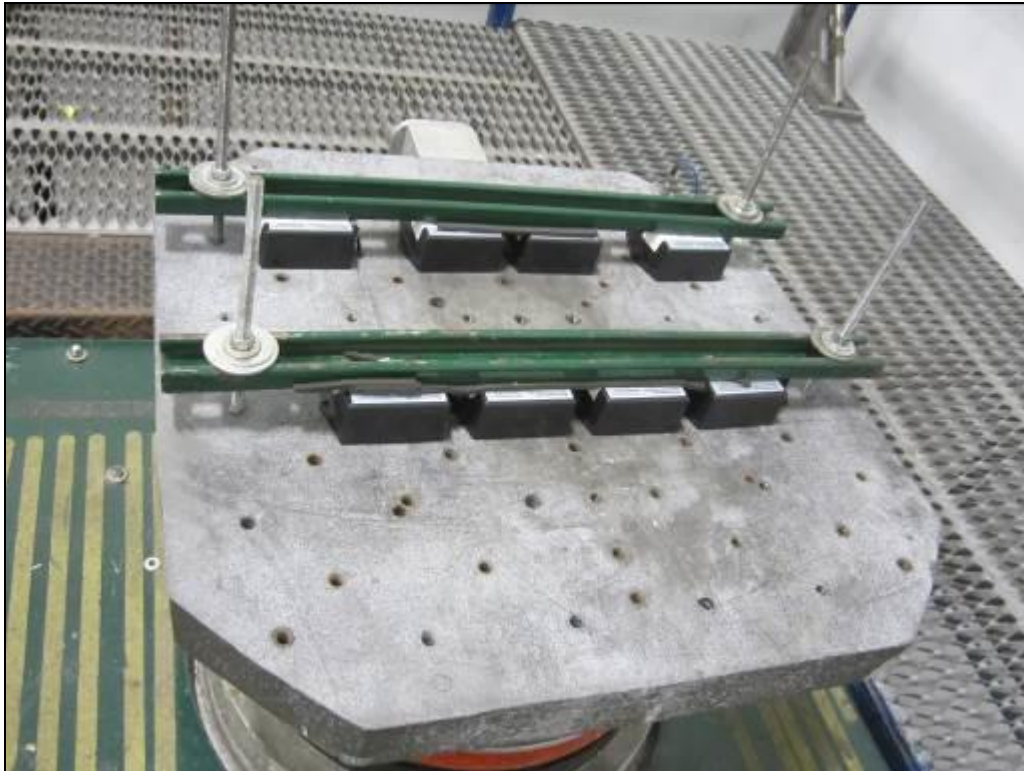
Photograph 10: Shock Test Setup – Vertical, Positive Direction
