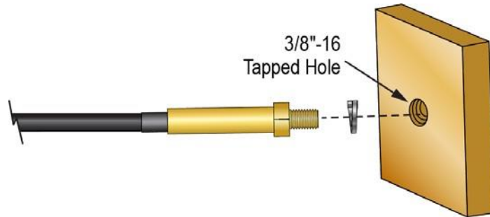
HPS Stud-Mount Temperature Sensor Installation
