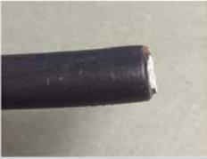
**Step 2: Cut and strip** (Extend the Coaxial Cable beyond the body of the stripping tool, after stripping, check and center conductor length. Reference the Pin Termination Table on Page #: 4
