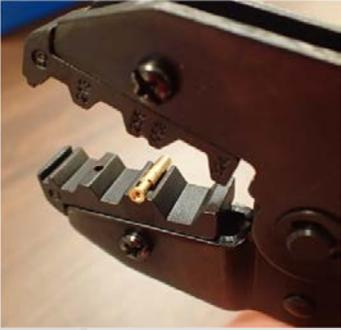
Place the pin in the correct crimp jaws
