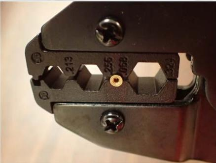
Close the crimp tool to barely hold the pin
