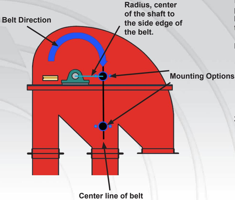
It is optimal if the sensor can be placed on the exiting side of the pulley (See arrow above for belt direction) on both the head and the boot.
