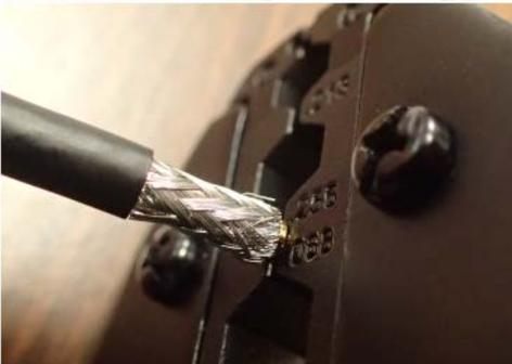
Fully Insert the conductor into the pin, then crimp the pin
