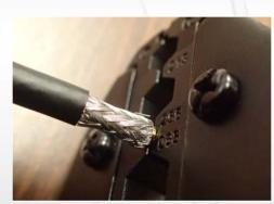
Fully Insert the conductor into the pin, then crimp the pin
