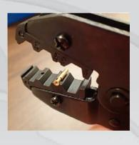
Place the pin in the correct crimp jaws
