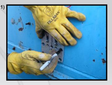
When mounting the belt alignment sensor, you will need a space greater than or equal to 1/4" from the belt to the sensor. If the belt rubs on the sensor it will damage the sensor. This may require the belt to be aligned prior to installation.
