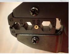
Close the crimp tool to barely hold the pin
