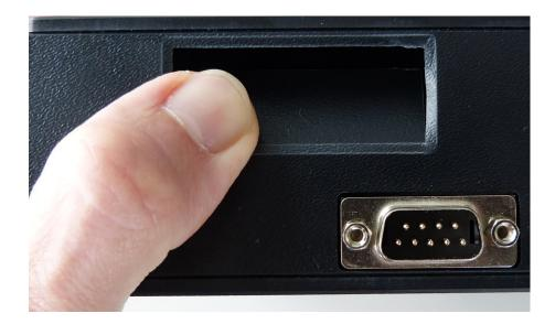
3. Flap the cut-out piece to the exterior with a small screw driver.
