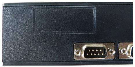
2. Carefully press to the upper side of the predetermined cut-out until the edge breaks
