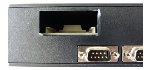
6. Insert the interface module carefully.
