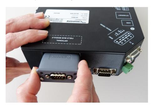
7. Tighten the two locking screws with a TORX 8 screwdriver
