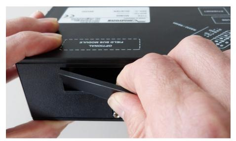
5. The mounting slot for the interface module is now ready for use
