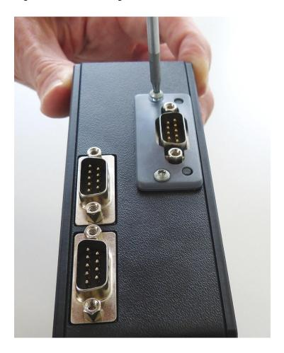
8. If you remove the interface module and leave the mounting slot empty, please cover the slot.
