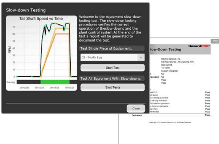
HazardPRO system managers have built-in slow-down testing. These convenient equipment slow-down tests can be performed from the control room. Slow-down testing simulates an equipment slowdown and allows you to confirm that your system warnings and shutdowns are operating properly. Once the slow-down test is started and the emergency threshold is reached the equipment will be shutdown.
