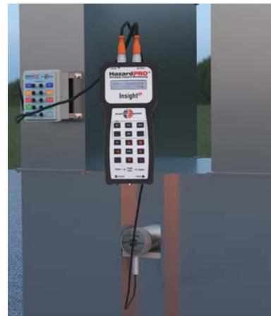
Insight<sup>HP</sup> connects to an elevator speed sensor to test for proper operation
