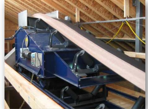
Tripper cars are instrumental to grain storage. Tripper cars provide unique opportunities for hazard monitoring as the movement makes Class II Div. 1 monitoring difficult. **HazardPRO** wireless sensors can be mounted directly to the tripper car, providing monitoring for speed, temperature and alignment. Wireless hazard monitoring provides a solution to the most difficult equipment to be monitored in your facility.
