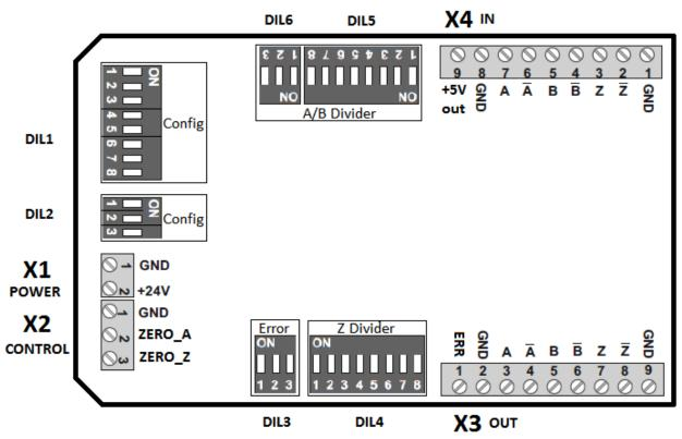
The green LED signals operational readiness (power switched on). The yellow LED signals an input error. (RS-422 or HTL Differential only) An HTL Error Signal (input error, only for RS-422 or HTL differential) is available on the X3 screw terminal 1. (Error = low) Basic settings:
