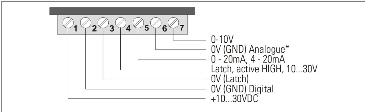
\* Potential separated from GND digital/ power supply (terminal 2)
