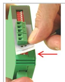
$\underline{\text{Switch position 1}} \text{ is responsible for } \underline{\text{all channels of Input 1}}$
