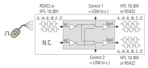
Input 1 is used as encoder input, and Input 2 remains unconnected. The input can be set to either symmetric (differential) format using A, /A, B, /B, Z, /Z channels, or to asymmetric (single-ended) format using A, B, Z channels only.
