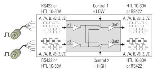
Both inputs can be individually set to either symmetric (differential) format using A, /A, B, /B, Z, /Z channels, or to asymmetric (single-ended) format using A, B, Z channels only. Acceptable input levels are RS422, TTL and HTL 10-30 volts.
