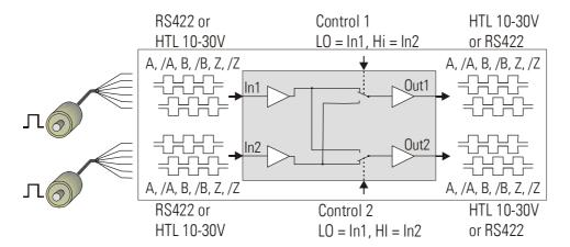
Both inputs can be individually set to either symmetric (differential) format using A, /A, B, /B, Z, /Z channels, or to asymmetric (single-ended) format using A, B, Z channels only. Acceptable input levels are RS422, TTL and HTL 10-30 volts.
