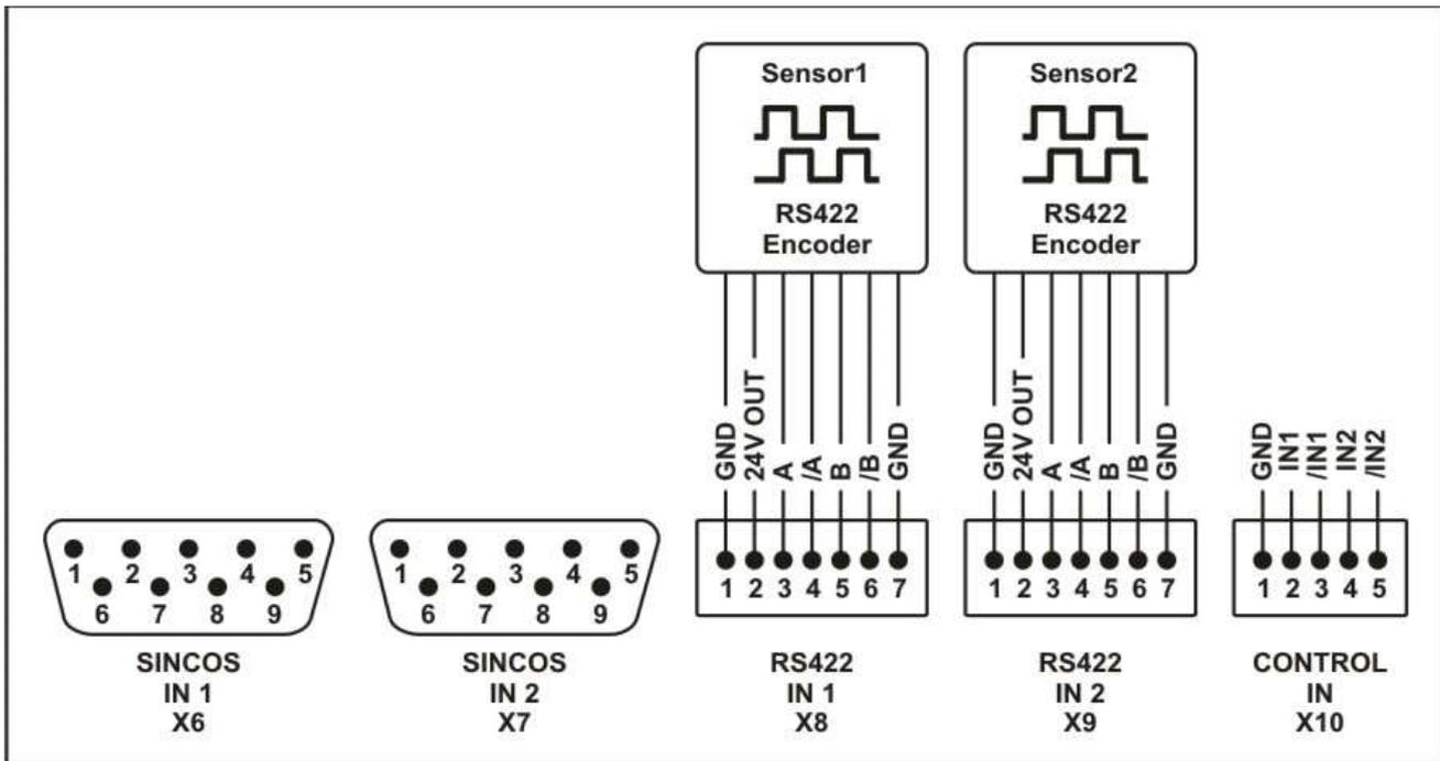
This mode (with DS23x models only) allows evaluation of a dual channel system, equipped with two identical RS422/TTL incremental encoders.
