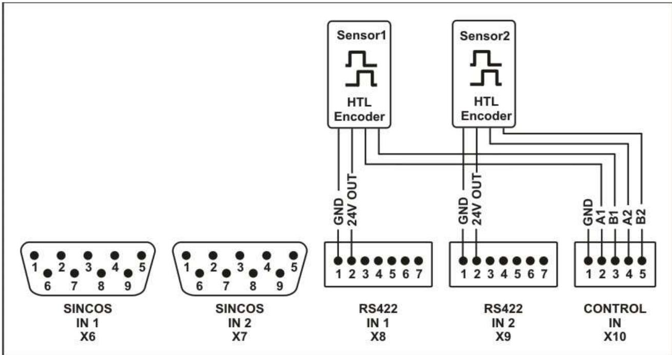
This mode allows evaluation of a dual channel system, equipped with two incremental dual channel HTL encoders.
