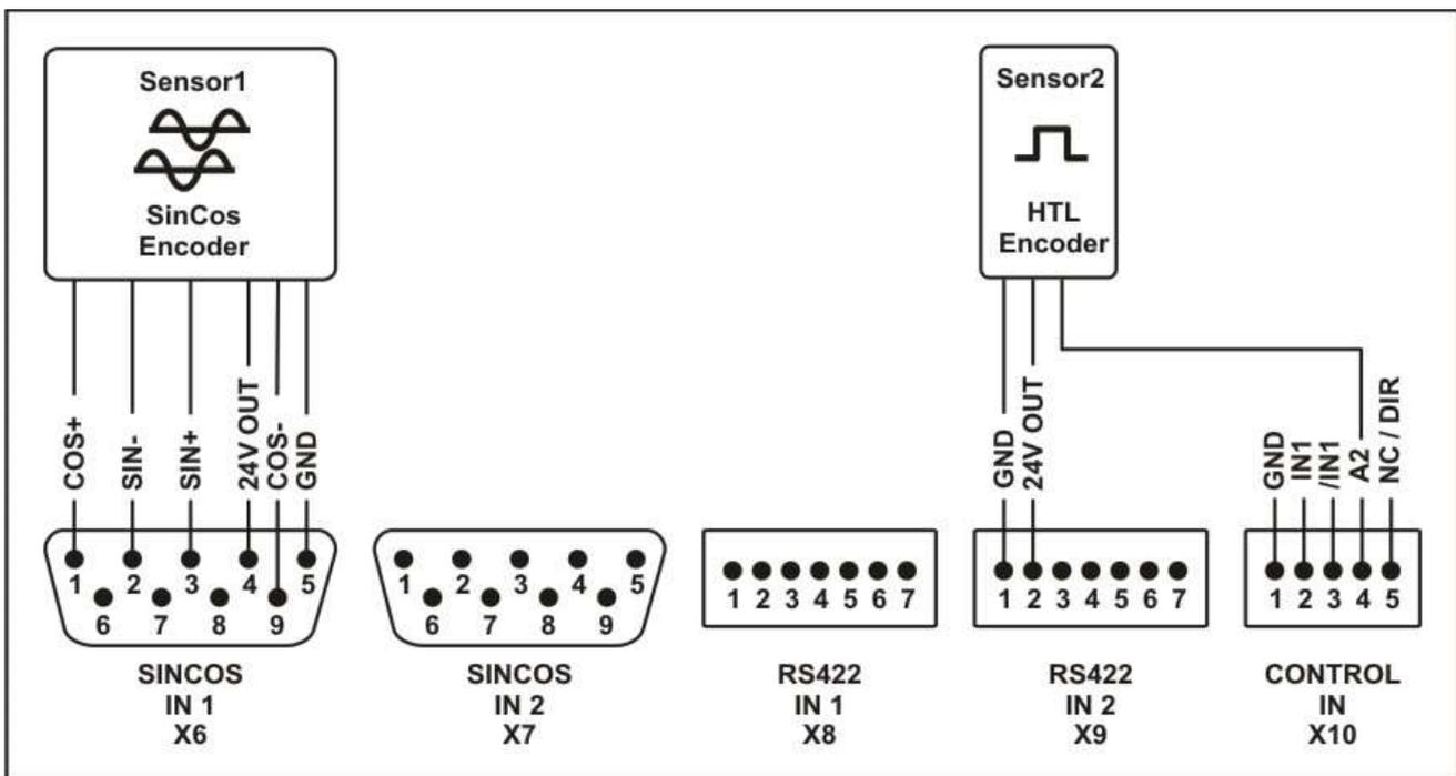
This mode allows evaluation of a dual channel system, equipped with a combination of one SinCos encoder and one incremental single channel HTL encoder.
