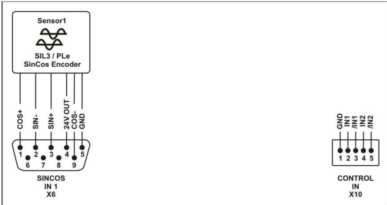
This mode is exclusively used for connection of a SIL3-certified or a PLe-certified SinCos sensor / encoder.
