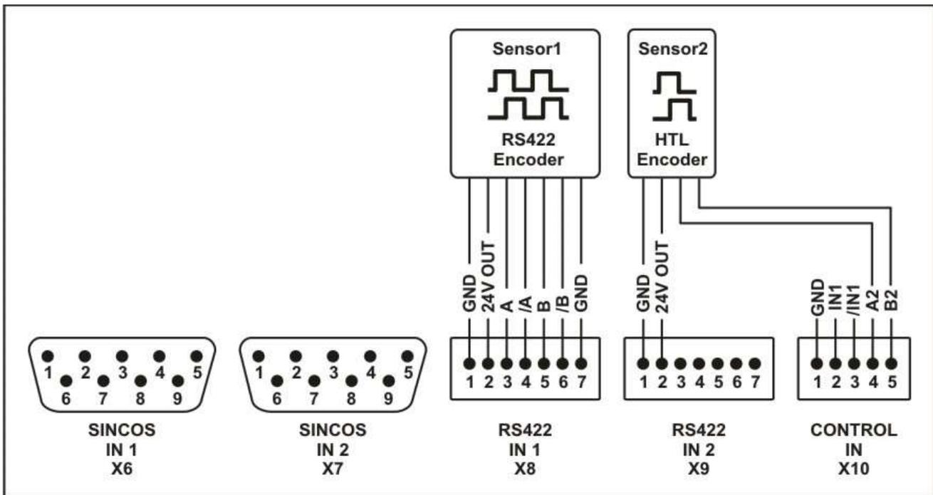
This mode is used for evaluation of a dual channel system, equipped with an incremental RS422/TTL encoder and a dual channel HTL encoder.
