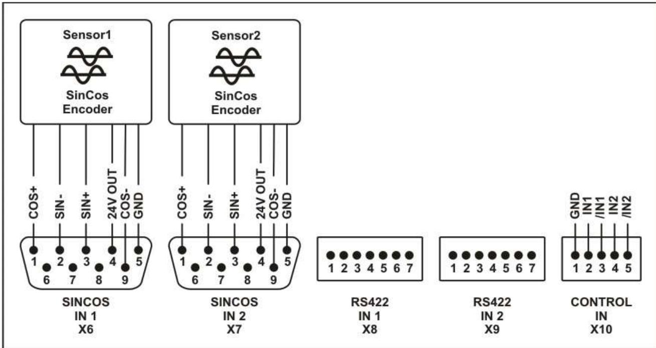
This mode is used to evaluate a dual channel system equipped with two SinCos sensors /encoders.
