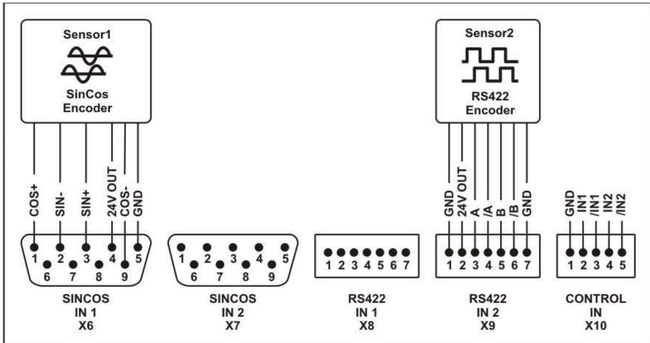
This mode allows evaluation of a dual channel system, equipped with a combination of one SinCos encoder and one RS422/TTL encoder.
