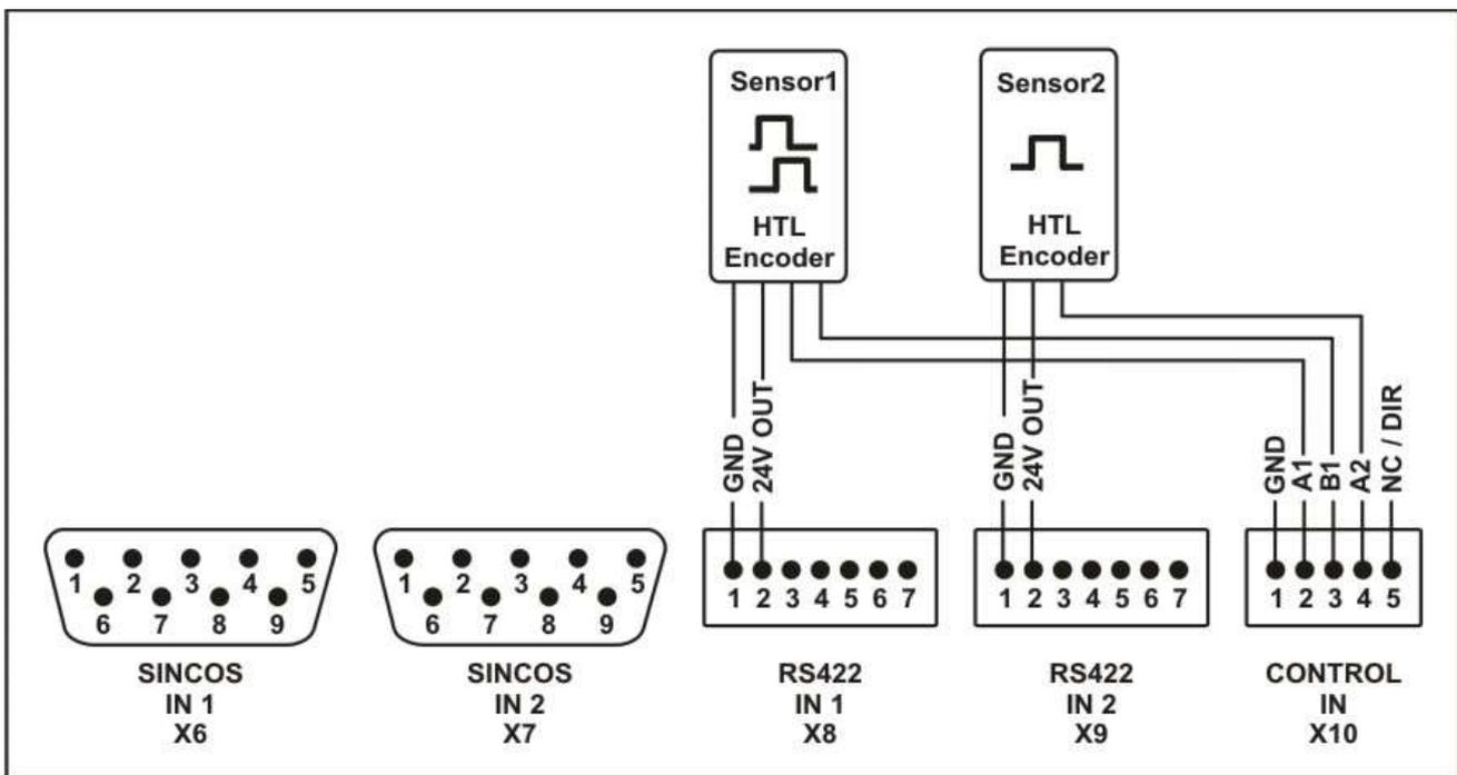
This mode allows evaluation of a dual channel system, equipped with a combination of one incremental quadrature HTL encoder and one single channel HTL encoder.
