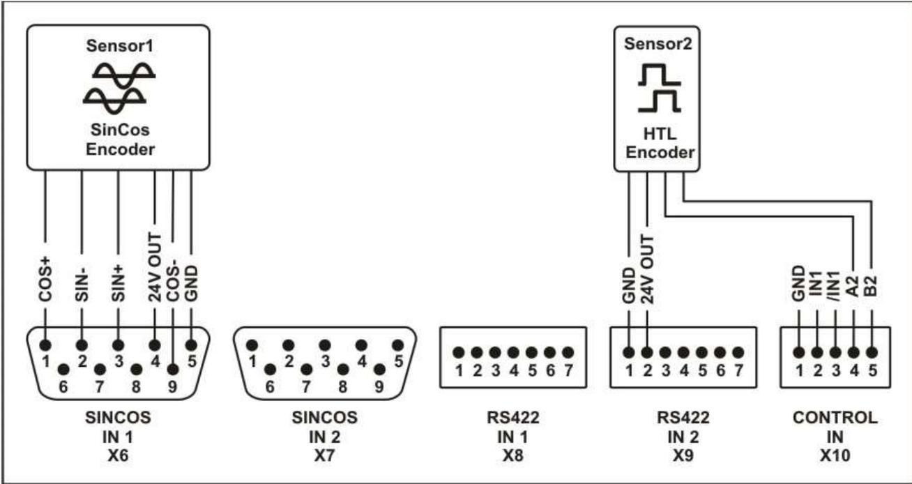
This mode allows evaluation of a dual channel system, equipped with a combination of one SinCos encoder and one incremental quadrature HTL encoder.
