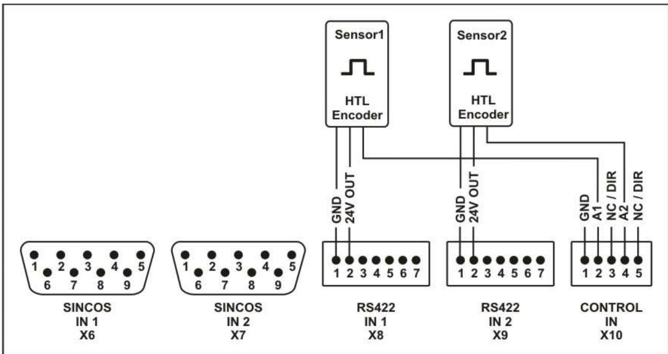
This mode allows evaluation of a dual channel system, equipped with two single-channel HTL encoders.
