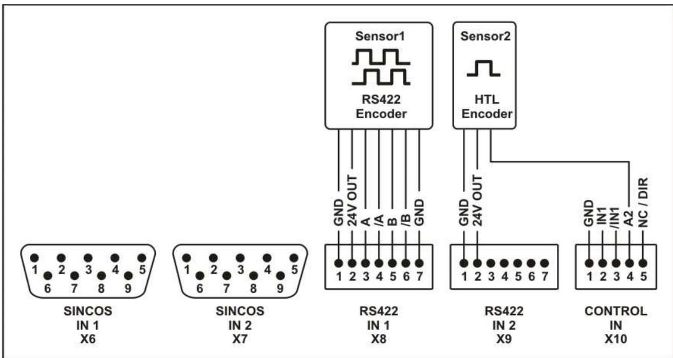
This mode (applicable with DS23x models only) is used for evaluation of a dual channel system, equipped with an incremental RS422/TTL encoder and a single-channel HTL encoder.
