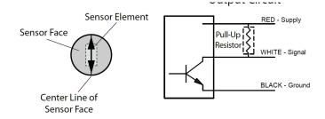
Note: Depending on the supply voltage, observe proper wattage rating of the pull-up resistor.
