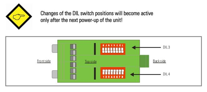
DIL switches **DIL3** and **DIL4** are located on the top side and switches **DIL1** and **DIL2** are located on the bottom side of the unit.
