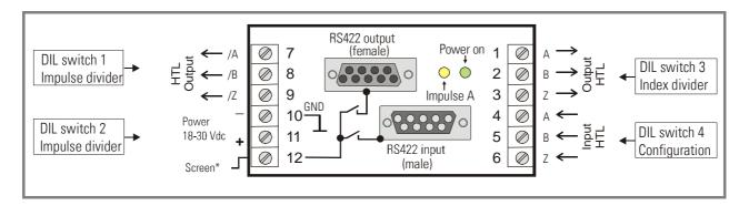
\*) This screen terminal allows to connect the metallic housings of the SUB-D-connectors to the potential applied to terminal 12 (e.g. PE or external GND or else), when the corresponding DIL switch is on (see settings of DIL 4 switch)
