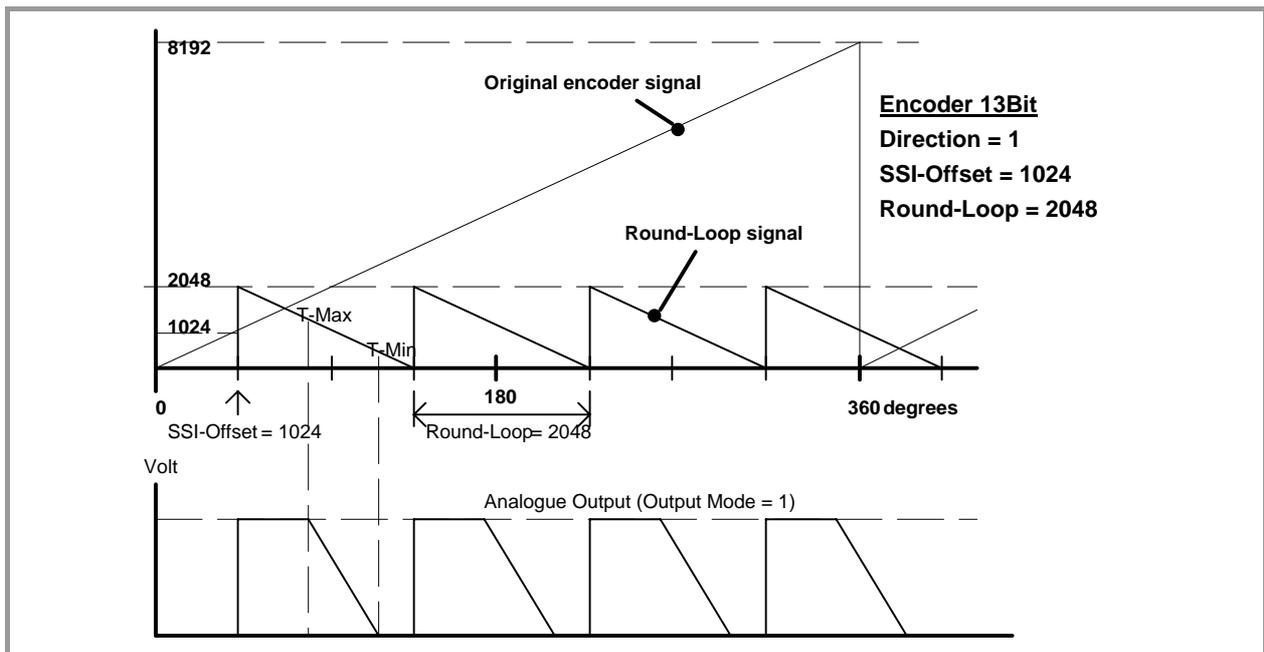
The Round-Loop function is also suitable to suppress the encoder overflow, when the mechanical zero position of your encoder lies between your Teach-Min and Teach-Max values and you do not like to change the mechanical situation. As shown in the subsequent picture, you need to set the Round-Loop register to the full encoder resolution and then shift the zero transition by setting the SSI Offset correspondingly.
