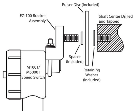
**Figure 8: EZ-Mount Bracket installation**
