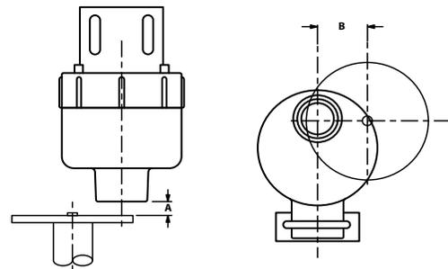
Figure 1: Speed Switch with 255 Pulser Disc
