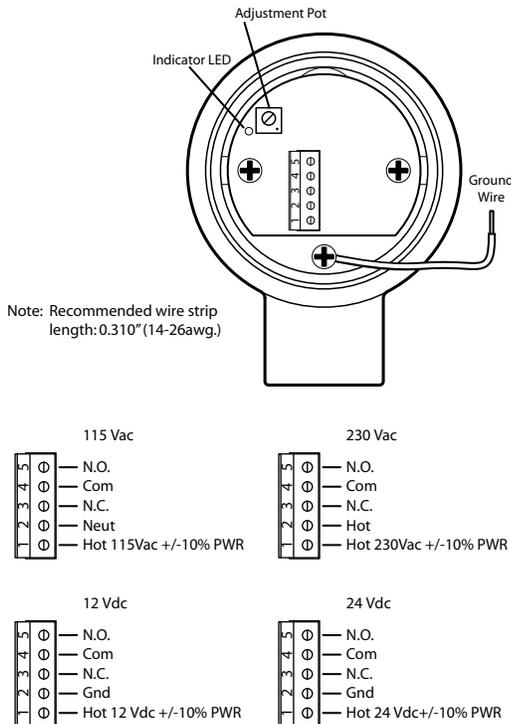
Figure 3: Set Point Adjustment
