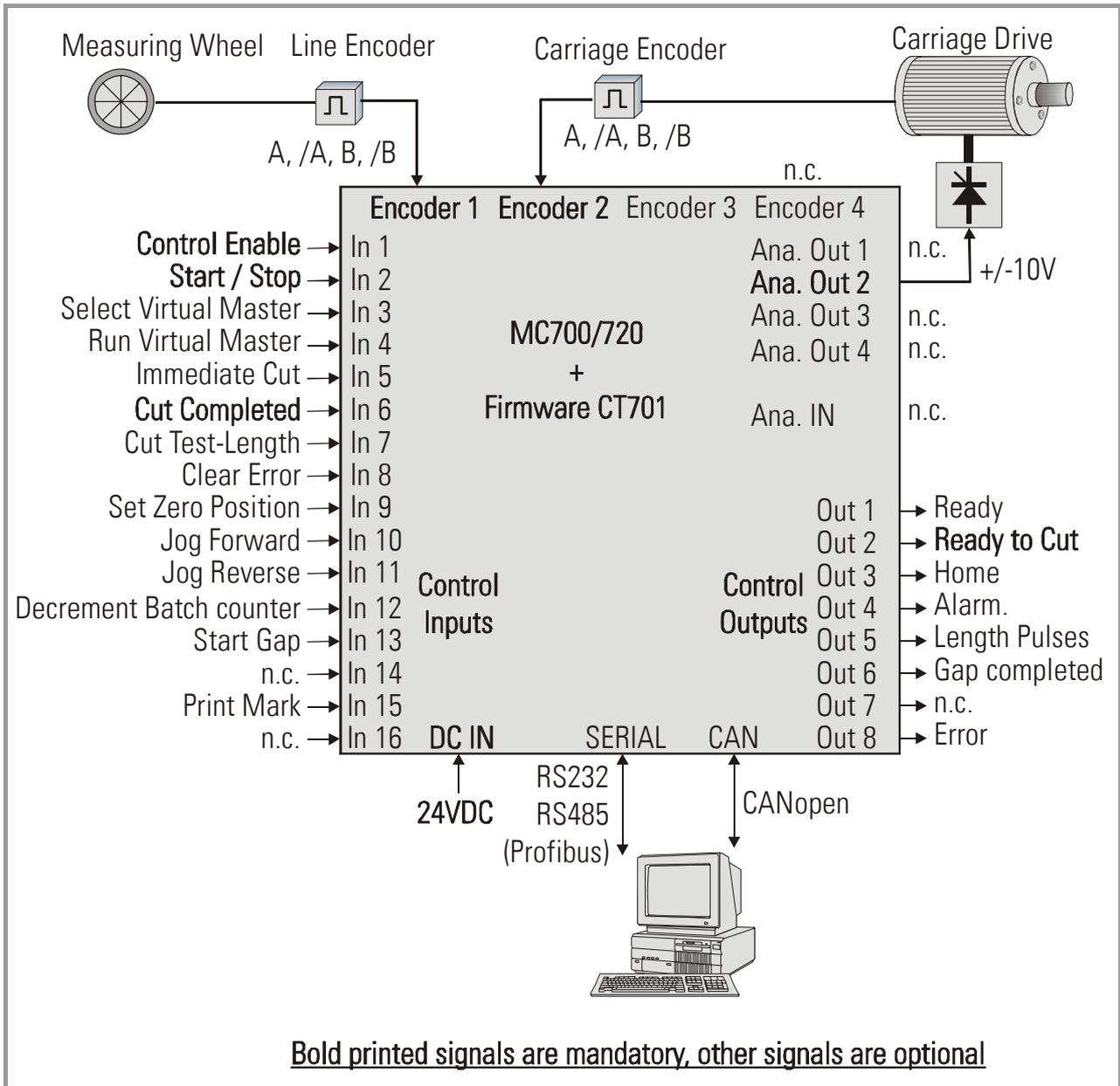
It is necessary to adjust the carriage drive to its maximum dynamic response (no internal ramps, no integral control loop, high proportional gain), because the FS701 will generate the ramps which the drive has to follow with no additional delay
