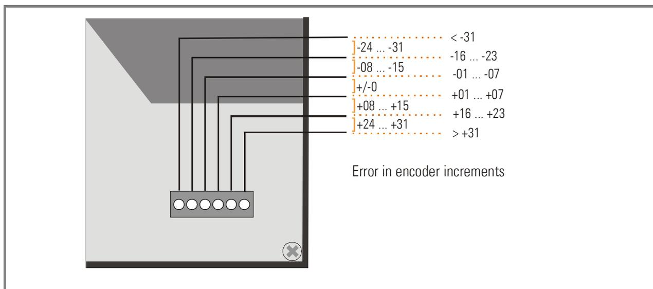
Positive errors (LEDs on right side of centre position) indicate that the carriage lags the line. Negative errors (LEDs on left side of centre position) indicate that the carriage leads the line. Under regular production conditions and with good adjustment of the control loop, you should find between 2 and 4 of the centre LEDs on or blinking, which indicates at the same time that the cutting accuracy is fine.
