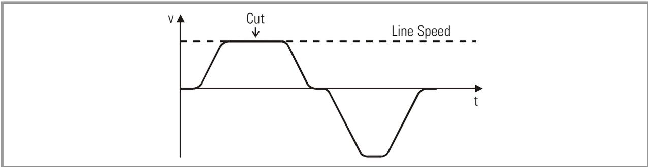
The FS701 control continuously measures the line speed and calculates an anticipation value to start the carriage before the cutting length is reached. Thus the shear will exactly match the cutting position of the material upon completion of the acceleration ramp and no overshoot or oscillation will take place prior to the cut. This saves time and increases the cutting efficiency of the shear system considerably.
