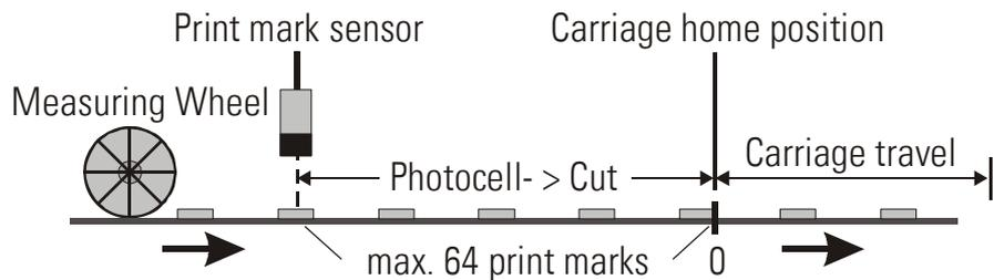
**Gap Length** With some applications it is desirable, after the cut, to produce a gap between following material and the piece actually cut, by short acceleration of the tool prior to removing it from its cutting position.
