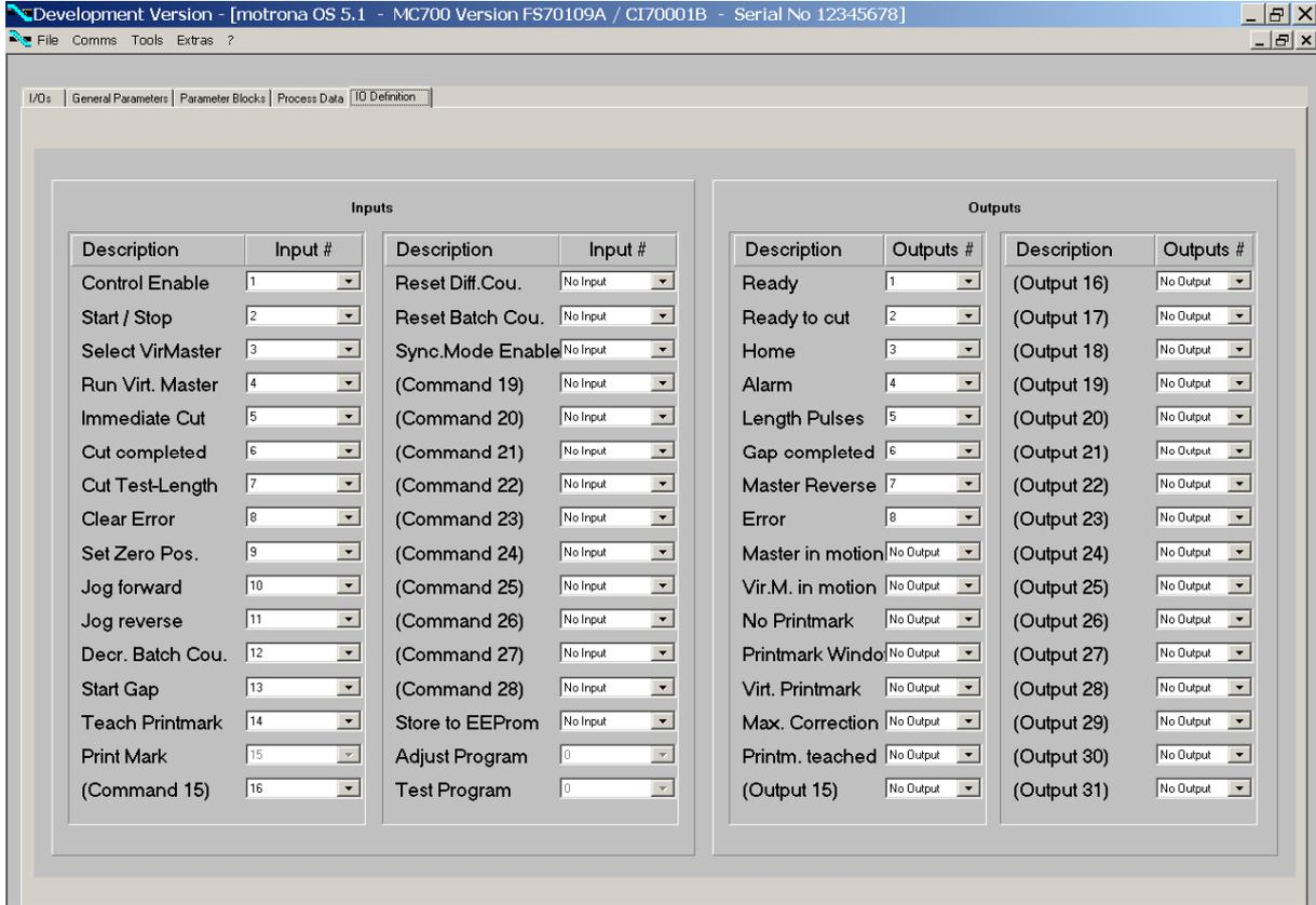
Any hardware input can be assigned to several input signals at the same time if necessary. The hardware input then switches all input functions associated in parallel.
