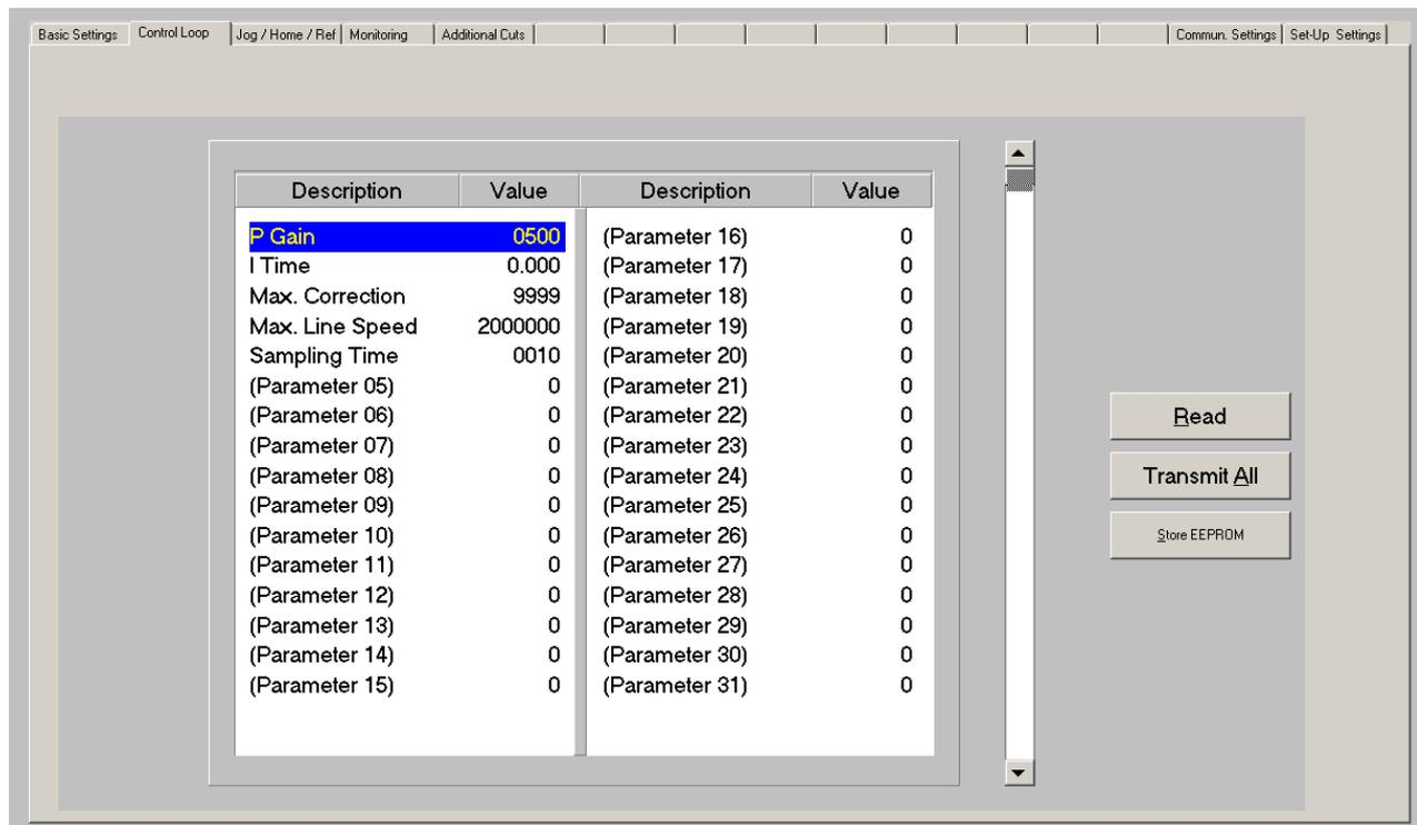
**P Gain** Proportional gain for compensation of relative errors of the carriage position with respect to the scheduled position.
