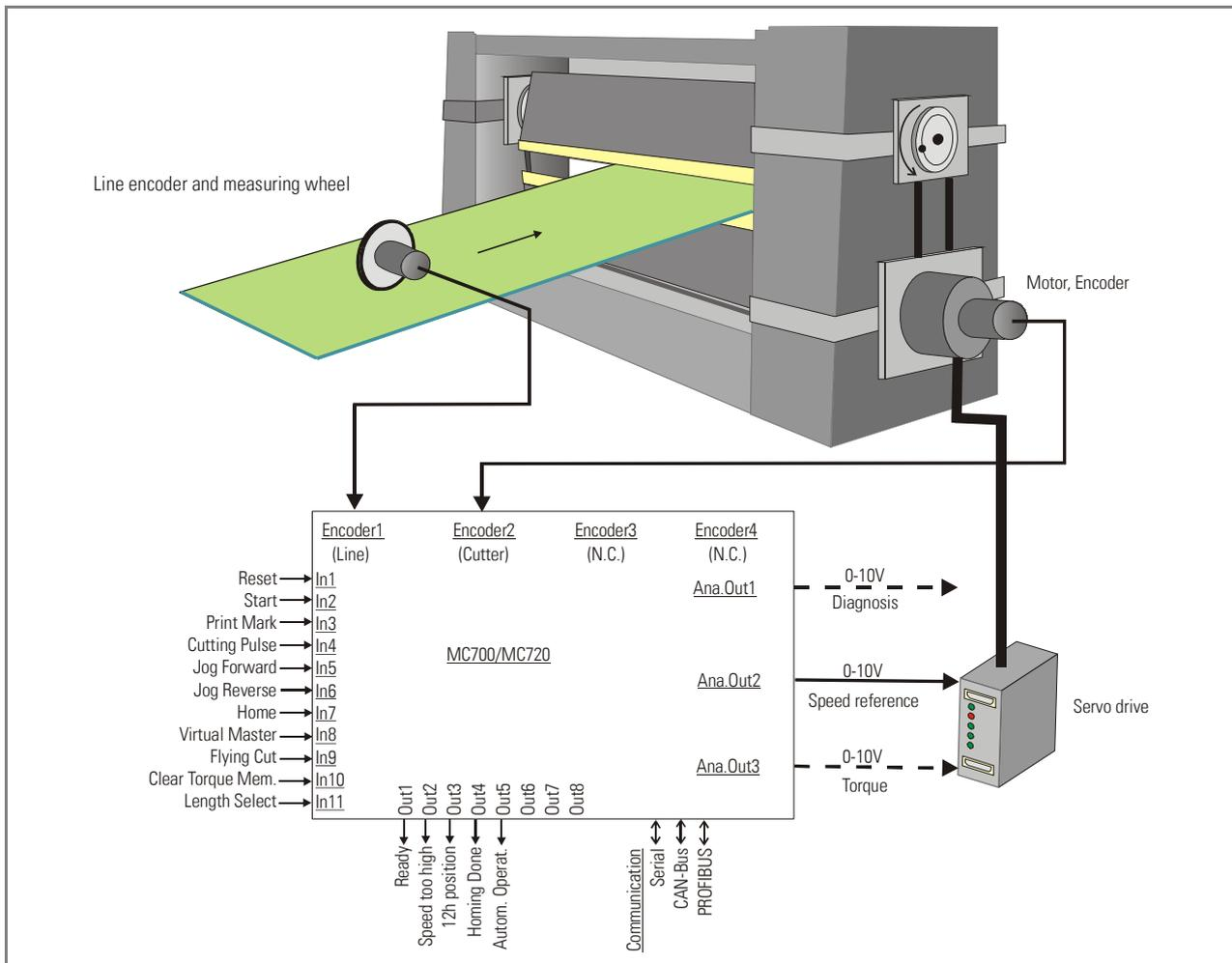
These cutting systems require the horizontal speed of the cutting tool to be synchronous to the material at any time of the penetration of the tool, whereas outside of the penetration zone, it is the cutting length and the active radius of the rotation that determine the speed profile.
