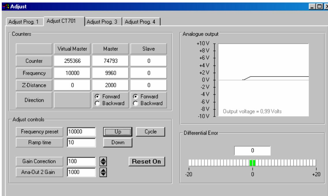
The Adjust Program is used to set the directions of rotation of the encoders and to adjust the analogue output with regard to the output level and the proportional Gain.
