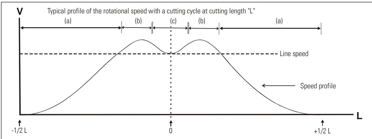
Zone (a) results from the ratio between the cutting length and the active rotating circumference of the tool.
