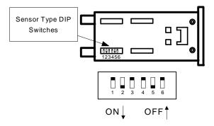
Figure 6; Sensor Type DIP Switches
