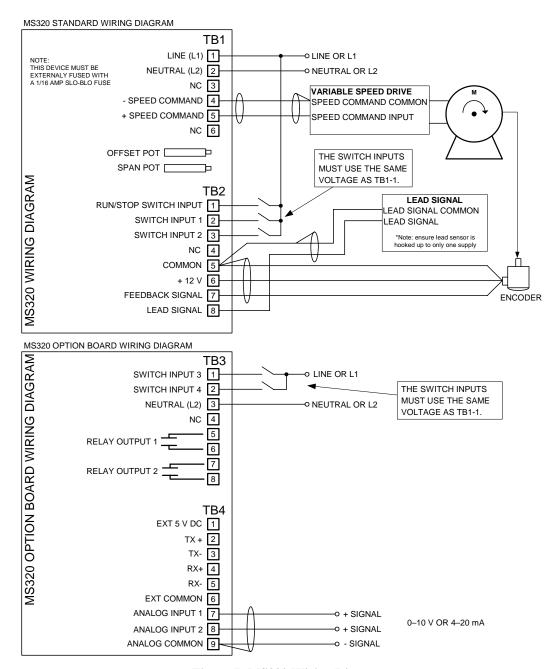
Figure 7; MS320 Wiring Diagram
