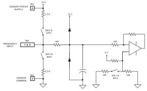
Figure 5; MS320 Sensor Input Circuit
