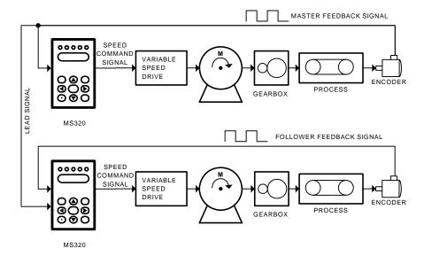
Figure 1; MS320 System Diagram
