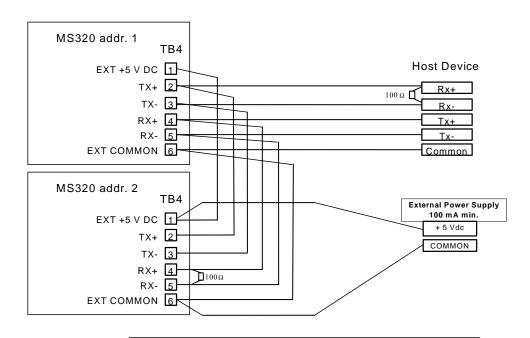
NOTE: 100 ohm terminating resistors should be placed between the Rx+ and Rx- terminals of the host device, and between the Rx+ and Rx-terminals of the last physical device on the communications network.
