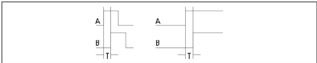
DIL switch S1 permits selection of 5 different times. The frequency is shown in brackets at which the phase displacement corresponds to 90°.
