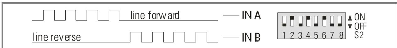
This mode of operation requires that one of the two inputs is in Low state while the other input line receives the pulses.
