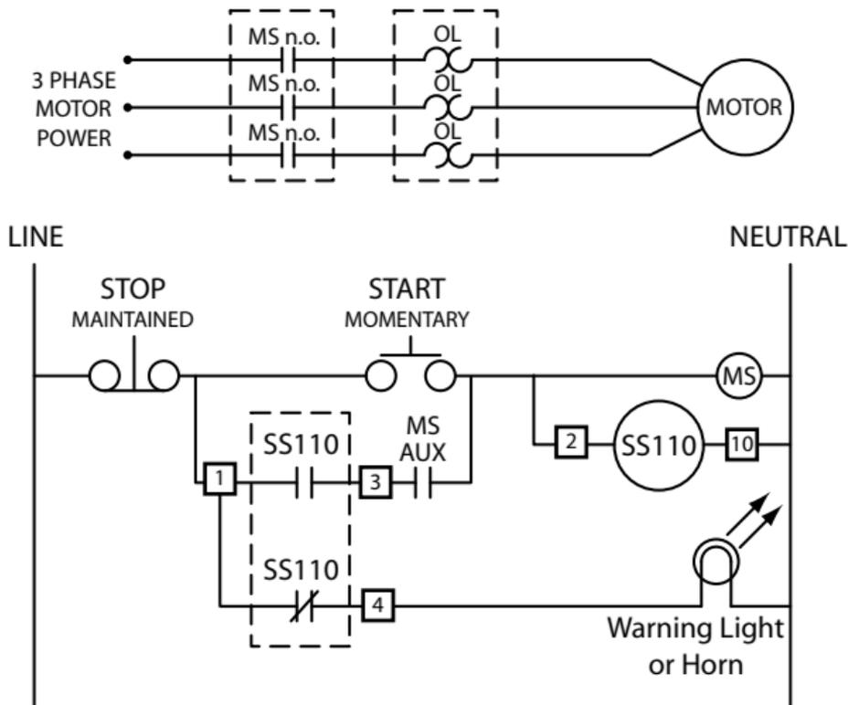
**Figure 7: Typical Wiring Diagram**
