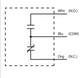
The relay output is electrically isolated from the VS1 DC power inputs and case
