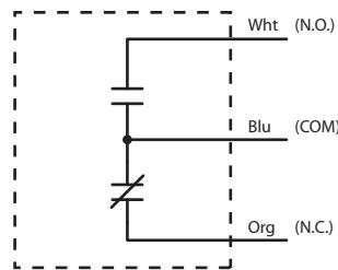
The relay output is electrically isolated from the VS2 DC power inputs and case
