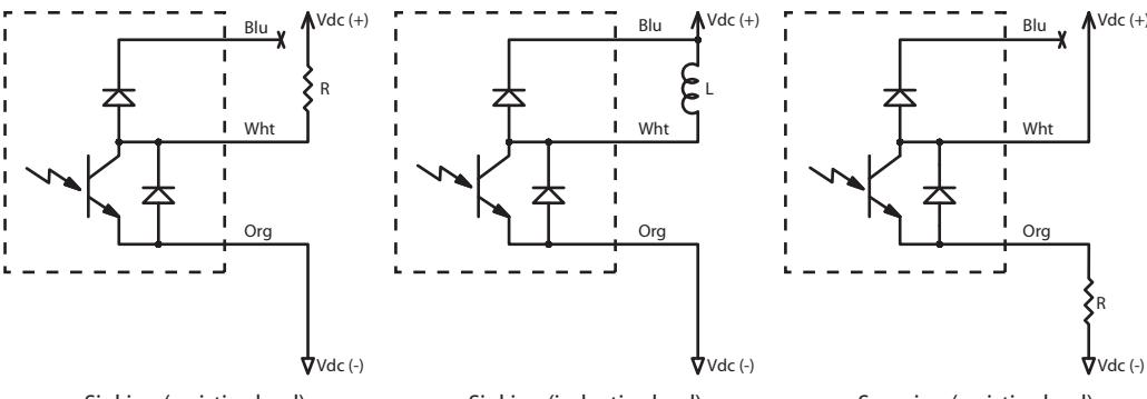
The NPN output is electrically isolated from the VS2 DC power inputs and case. The NPN output may be externally connected to the same supply as the DC power inputs or to a different supply.
