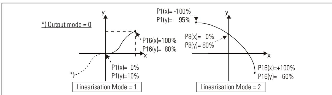
You can visualize your curve on the PC screen or by means of an external oscilloscope. For this, select TOOLS, then TEST and there „Analogue Voltage Function“. The unit will now simulate a repeating counting cycle over the full range and generate the analogue signal accordingly. When you use the Scope function of the operator software, you must set the serial code „:1 “ to record the analogue output.
