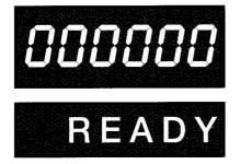
Upon power-up, the MicroLength 196 will display 0's (zeros) on the length display, and the alphanumeric display will read READY. This means the MicroLength 196 is ready to accept setup data, or to RUN at the previously programmed set point. After a variable is entered or a new operating length is set, the display will return to its READY state to wait for the RUN command.
