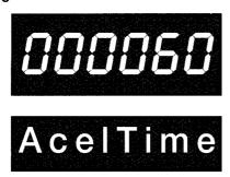
The variable changed in this example is Acceleration Time (variable #07). You would have selected 07 and pressed the ENTER key in the above example. The display shown here would appear. The alphanumeric display shows that Acceleration Time (Acel Time) is being set. The length display will show the last Acel Time entered. To enter a new Acceleration Time, simply press the number of seconds desired from stop to full speed (.05 to 600 – in this example 60 seconds), and press the ENTER button.
