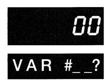
To set a variable, press the VAR key. The alphanumeric display requests a two-digit variable number and the speed display shows two zeros, which will "echo" the variable selection. Simply press the variable number and then the ENTER key. If you are unsure which variable number to enter, press the up/down arrow keys to scroll through the menu of variables. When the variable you want to change is displayed, press the ENTER key.
