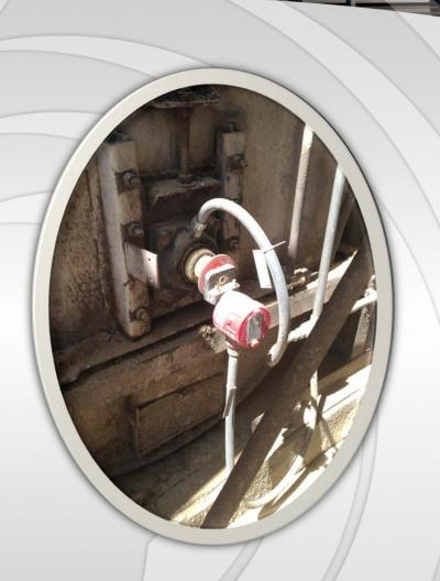
FB420 Speed Sensor with relay monitoring speed on a grain elevator (with EZ-100 Mount and EZ-255 Pulser Disc
